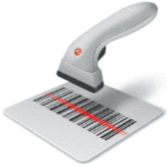
It is also known as a POS (point of sale) scanner. The bar code reader scans the bar code image using light, which is then reflected and translated into an analog signal. The signals are then decoded and transformed into alphanumeric values to be stored in a computer connected to a barcode reader. This ultimately helps in identifying product details and prices from the database
